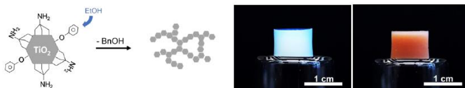
FIG. 1. Schematics of the solvent-triggered self-assembly process and images of the synthesized TiO 2 and TiO 2 /MagPlas NWs
